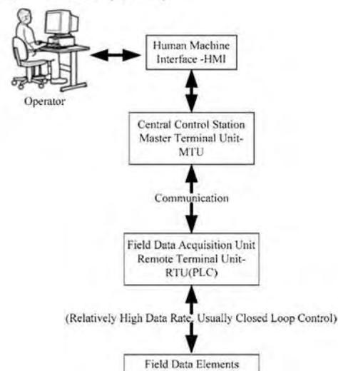
Fig. 1 SCADA System Architecture
