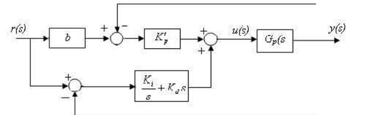
Fig. 3 Implementation of PID control for integrating and unstable Processes
