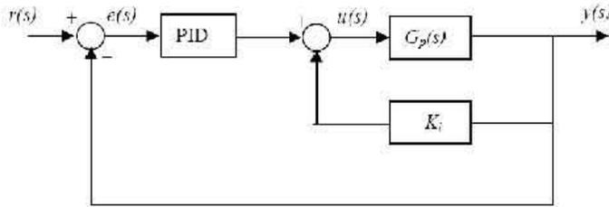
Fig. 2 Block diagram of two loop controller
